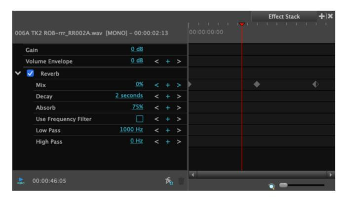
Keyframes can be created on parameters in the effects stack. They can be visualized and manipulated from the right part of the effect stack.
