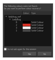
**Colour Recovery**: By default, if a colour palette required to display a drawing is missing because it has been moved or deleted, Harmony recovers the missing colours into a new temporary palette. If this option is disabled, Harmony will skip this step and display the zones painted with missing colours with the Replacement Colour, which is solid red by default.
