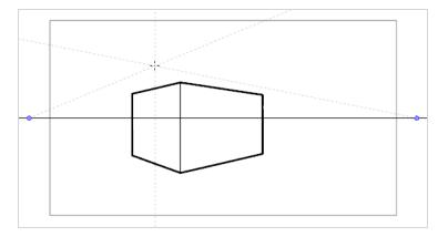
• The **3-Point Perspective (Bird's Eye View)** guide helps you draw lines coming from one of three vanishing points. Like with the 2-Point Perspective guide, two vanishing points are placed on the horizon line, which are used to draw horizontal lines on either the x-axis or the z-axis. The other vanishing point is placed below the horizon line to help draw lines on the y-axis.
