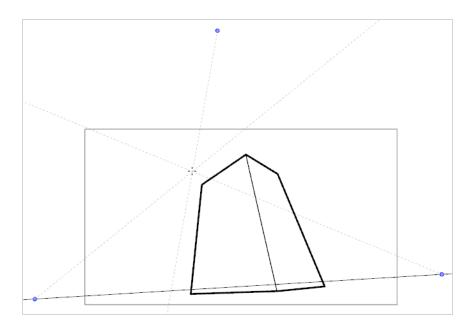
• The **3-Point Perspective (Horizontal Pan)** guide helps you draw horizontally panoramic backgrounds, with curvilinear horizontal lines. A vanishing point is placed in the middle of the horizon line, to help draw lines on the z-axis, and two vanishing points are placed on the horizon line outside of the camera field, to define the curve of the horizontal lines. Vertical lines are made perpendicular to the horizon line.
