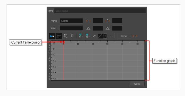
This dialog will allow you to animate the function. The function graph at the bottom is made to represent the values of the function throughout each frame in the scene.
