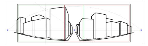
• The **3-Point Perspective (Vertical Pan)** guide helps you draw vertically panoramic backgrounds, with curvilinear vertical lines. A vanishing point is placed in the middle of the horizon line, to help draw lines on the z-axis, and two vanishing points are placed above and below the horizon line, outside of the camera field, to define the curve of the vertical lines. Horizontal lines are made parallel to the horizon line.
