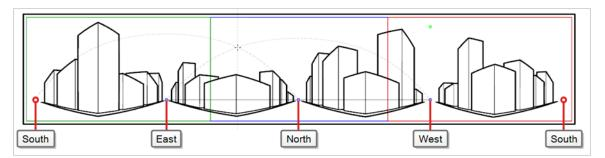
• The **4-Point Perspective (Vertical Pan)** is a lot like the 2-Point Perspective guide, except that its vertical lines are curvilinear, so it can be used to make vertically panning backgrounds. Two vanishing points are on the horizon line, outside of the camera field, to help draw lines on the x-axis and the z-axis, and two vanishing points are placed above and below the camera field to define the curve of the vertical lines.
