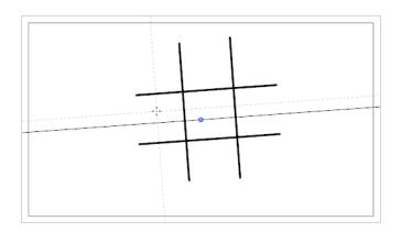
• The **Isometric Perspective** guide helps you draw lines that are parallel to one of three axes: The x-axis, the y-axis and the z-axis. The angle of each axis can be customized as needed.
