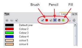
The Colour view can keep track of the colour you were using the last time you were using either the Brush tool, Pencil line tool (Pencil, Polyline, Line, Rectangle or Ellipse) or Paint tool.
